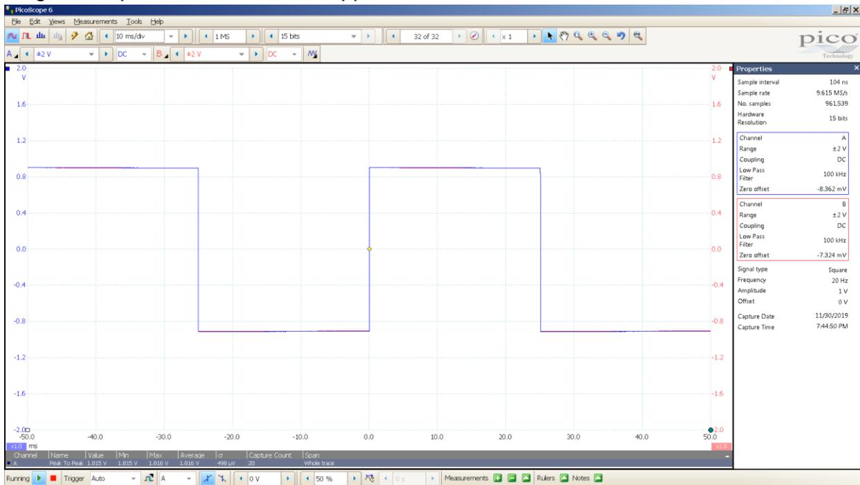
Magni 3+ square wave 20 Hz 2 Vpp 10 mS / div 32R load 5 MHz BW
