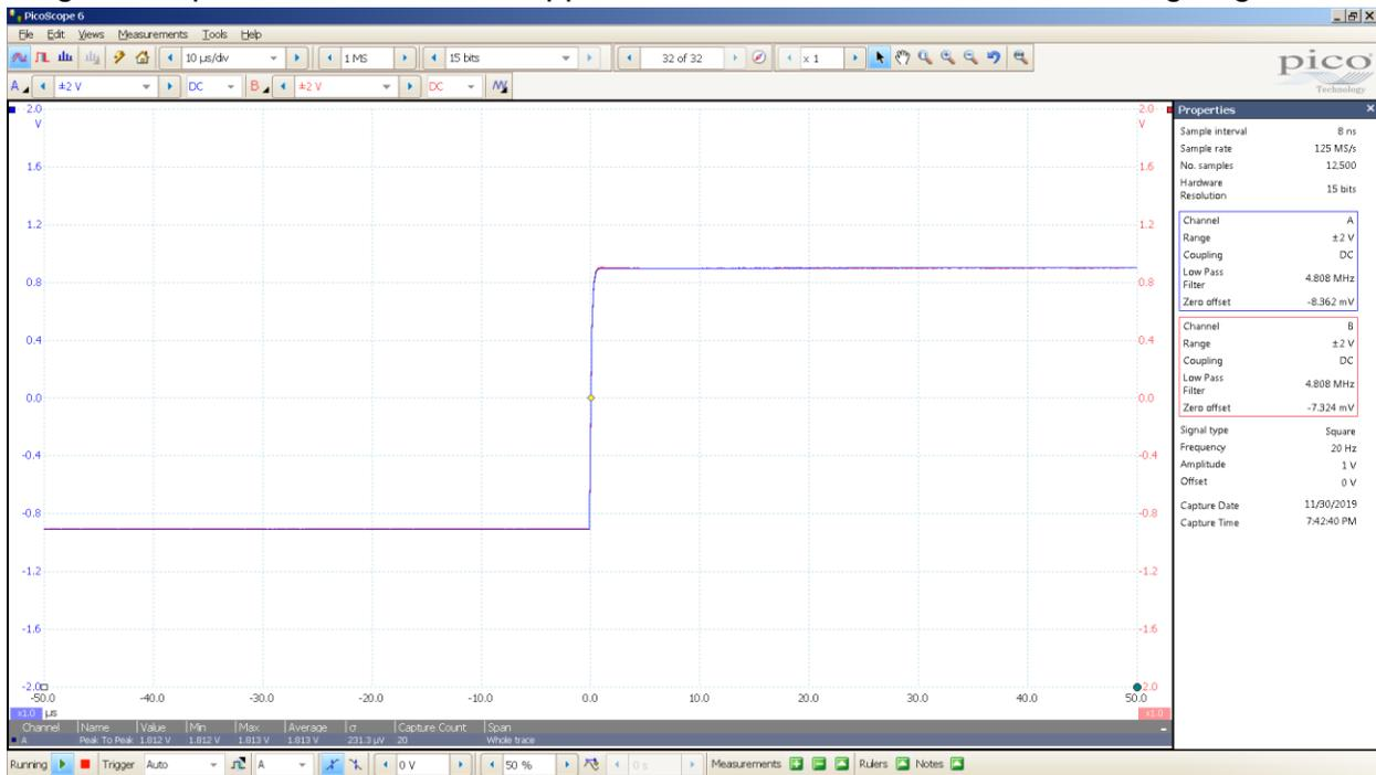
Magni 3+ square wave 20 Hz 2 Vpp 10 uS / div 32R load 5 MHz BW falling edge
