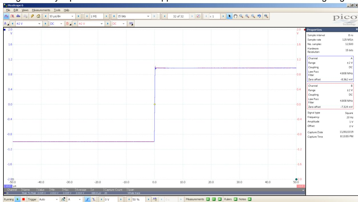
Magni Heresy square wave 20 Hz 2 Vpp 10 uS / div 32R load 5 MHz BW falling edge
