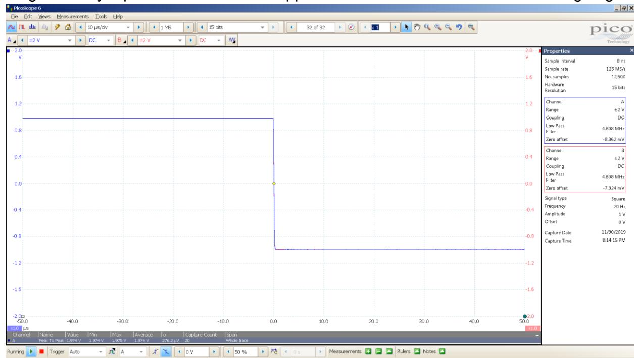
Magni Heresy SE input SE Output square wave measurements
