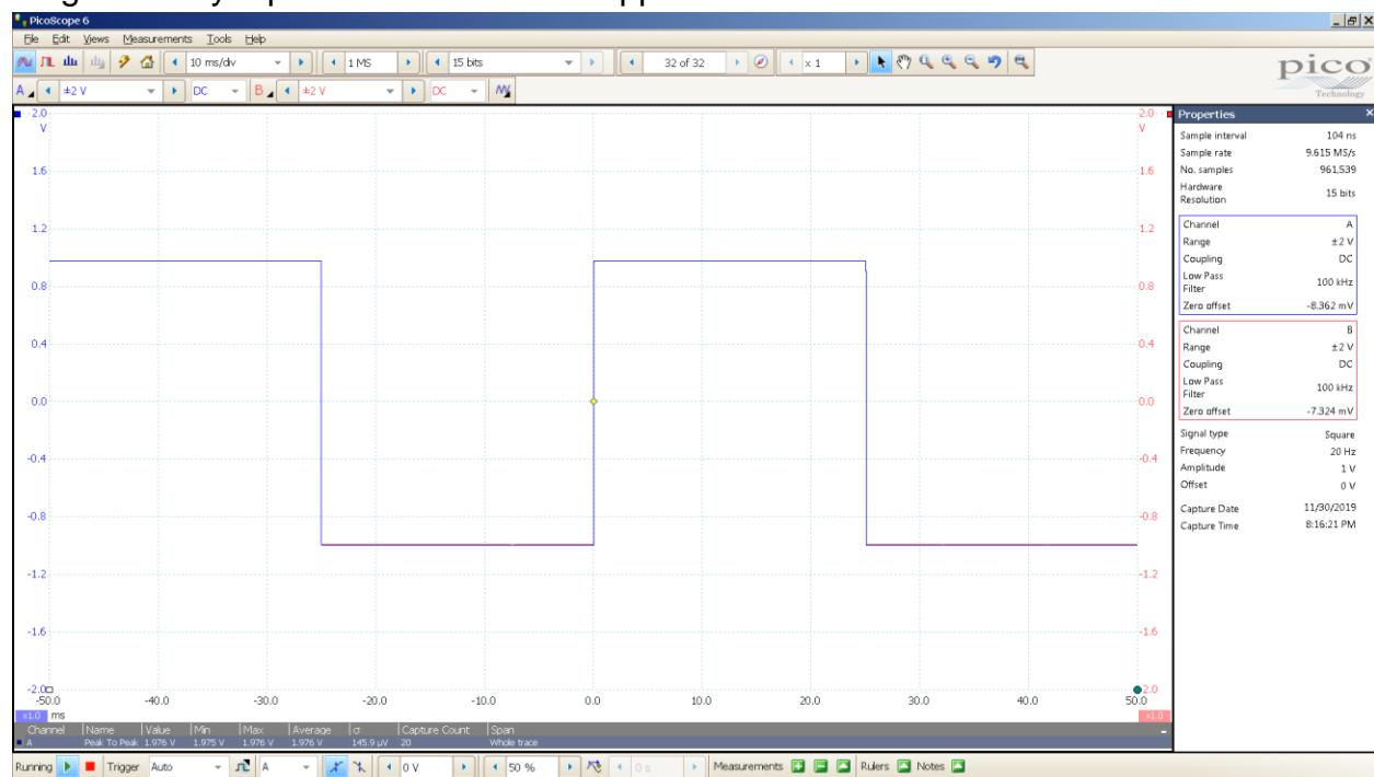
Magni Heresy square wave 20 Hz 2 Vpp 10 mS / div 32R load 5 MHz BW
