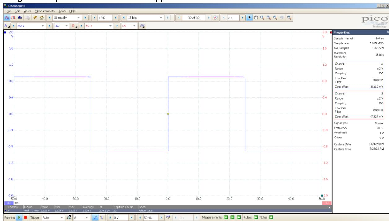
Magni 3+ square wave 20 Hz 2 Vpp 10 mS / div 300R load 5 MHz BW
