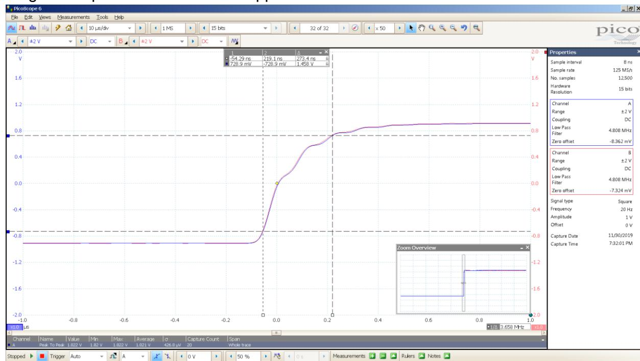
Bandwidth estimation:  $BW \text{ (MHz)} = 0.35 / RT \text{ (mS)}$
