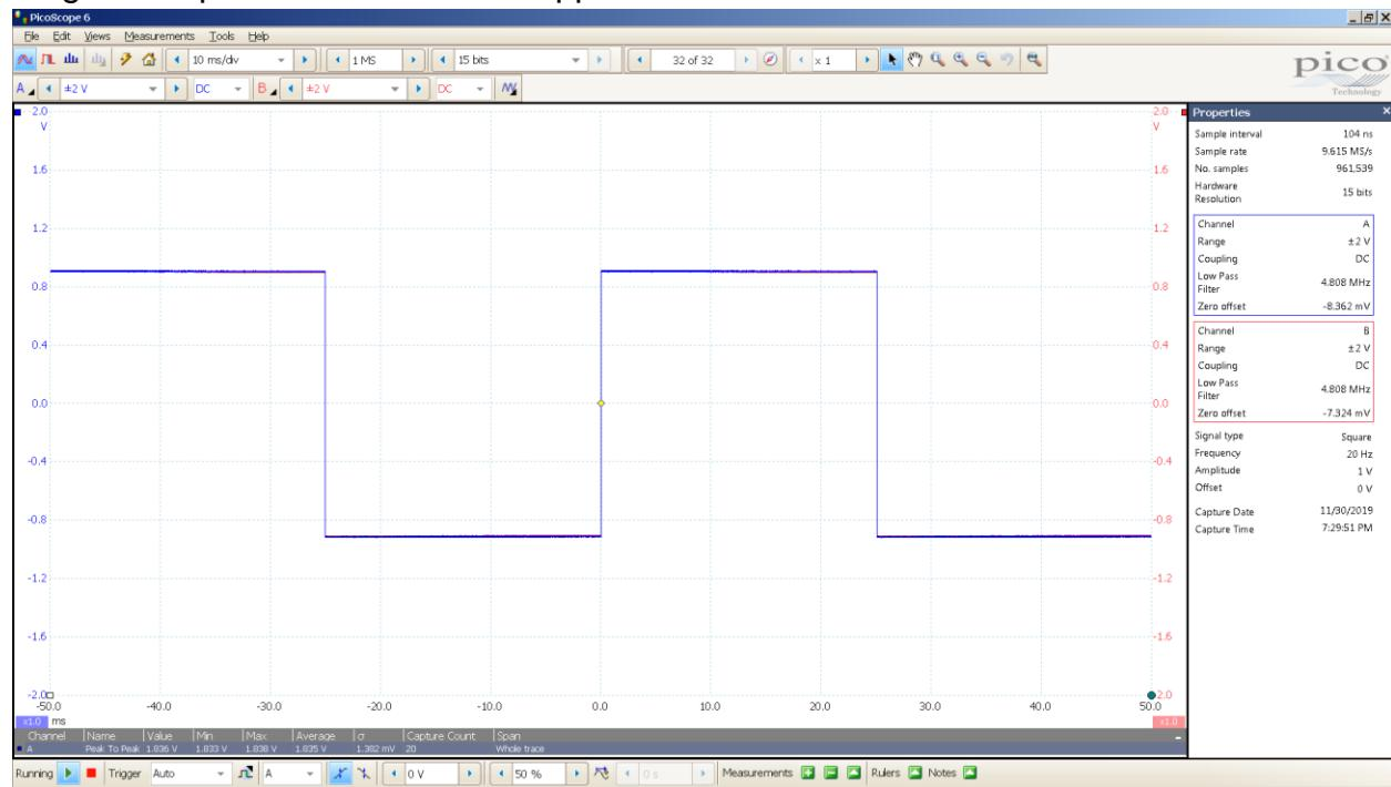
Magni 3+ SE input SE Output square wave measurements
