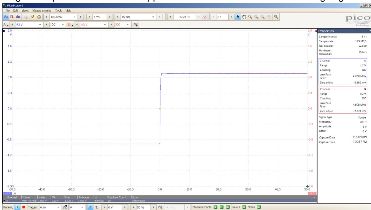
Magni 3+ square wave 20 Hz 2 Vpp 10 uS / div 300R load 5 MHz BW falling edge
